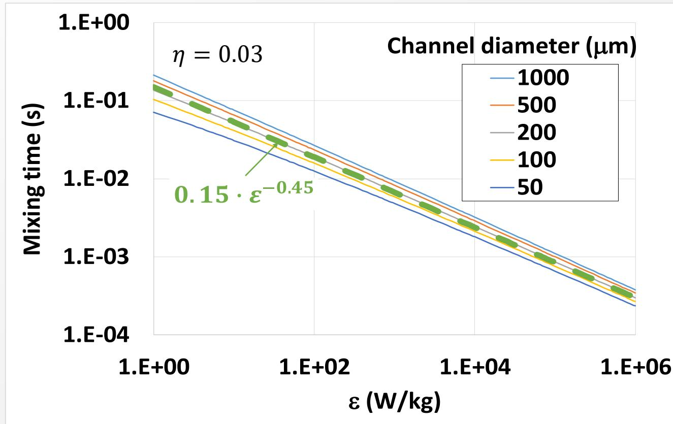
Data for channel diameters between 50 and 1000  $\mu\text{m}$  with  $\eta = 0.03$  : well described by power law  $t_{diff+shear} = 0.15 \cdot \varepsilon^{-0.45}$
